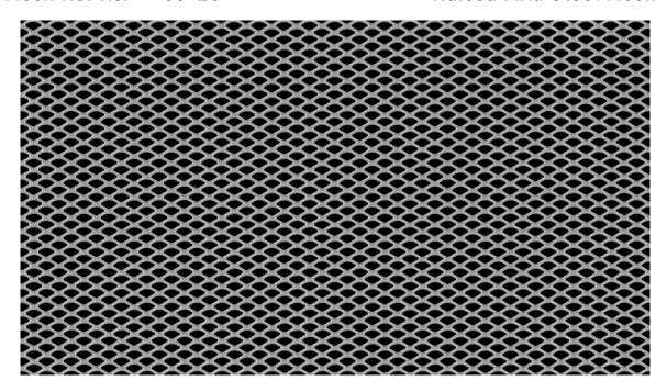
LW Pitch:6.00mmStrand Width:0.79mmSW Pitch:3.50mmThickness:0.60mmWeight:2.11 kg / m2Open Area:55%
